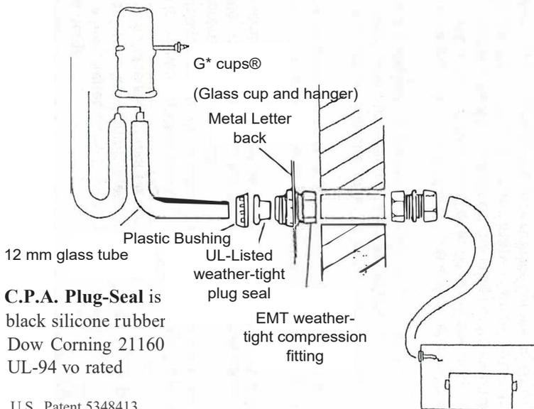
C.P.A. Plug-Seal is black silicone rubber Dow Corning 21160 UL-94 vo rated
